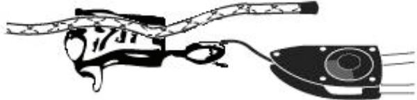
Position the clamp on the strand you are tensioning and attach the clamp to the "S" hook on the ratchet as shown.
