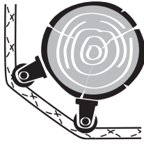
To reduce the potential for leg injuries, posts should remain outside the fence.
